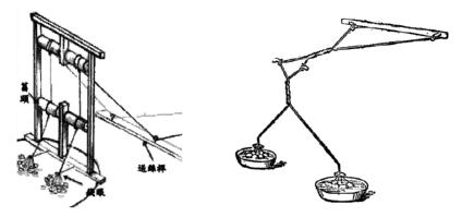
Fig. 5 a [left]: The croisure according to the description held in *Nongsang jiyao (futou* 菌頭: pieces for forming the *croisure*; *qianyan* 錢眼: guiding-eyes; *liansi gan* 連絲桿: pull-up lance)
